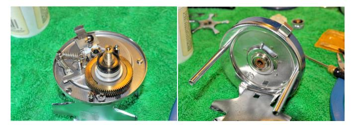
Replace the pinion gear and the main gear assembly-remember to put some grease on the main shaft where the gear contacts. Rebuild the gear stack in the correct sequence (check the disassembled photo if unsure). Replace the side plate lining up the notch on the drive shaft bearing casing (black plastic part) with the notch in the side plate. Replace the two bridge screws.
