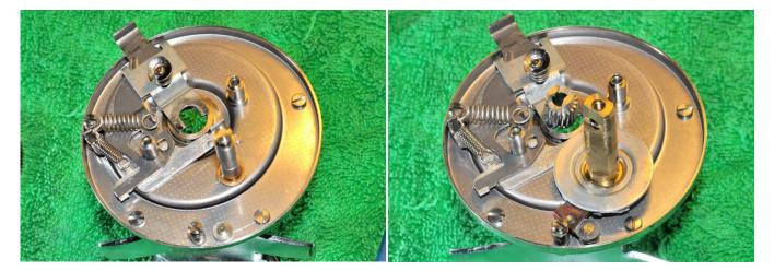
Replace the pinion yoke spring and the pinion yoke lock. Replace the press arm spring and the clutch spring. Add some oil to the gear shaft and then replace on the side plate-don't forget the anti reverse pawl.
