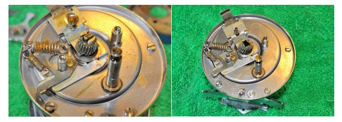
Remove the pinion yoke lock and the pinion yoke spring-take care as the spring is compressed and you need to make sure it doesn't fly off. Remove the pinion gear and the press arm spring (stronger spring ) and the clutch spring (weaker spring).
