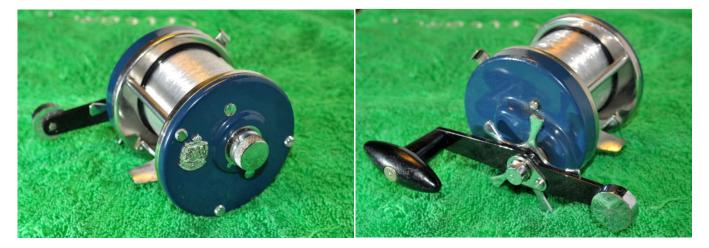
This is a single speed reel and so servicing is pretty straight forward. Mechanically this reel seemed fine although the drag was very sticky and the gears felt as if they needed a lube.
