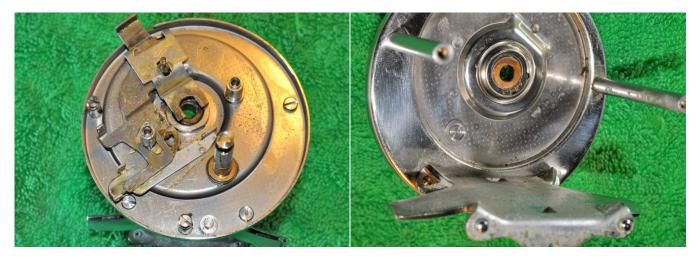
Remove the free spool press arm, free spool clutch and the pinion yoke. Access to the bushing is on the other side of the side plate. Remove the circlip and the bushing. Giving the bushing a good clean and then flood with oil.
