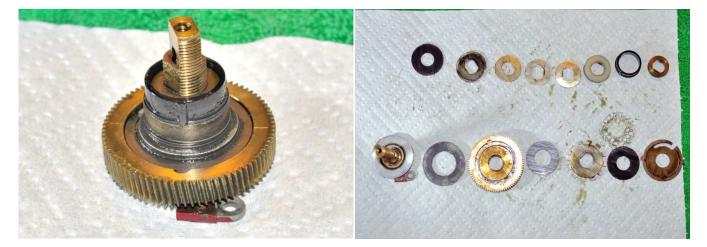
Lift off the whole gear assembly and anti reverse pawl and then separate it out. In the photo bottom left is bottom of the assembly and top right is top of the assembly. Note that there is a shim that sits under this assembly-it is still on the brake plate in the photos below.
