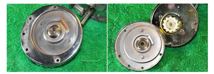
To access the bushing on the left side plate you need to undo the two screws on the inner plate-these are held captive in the side plate. The bushing on this side is also held in place with a circlip-again clean thoroughly and then flood with oil.
