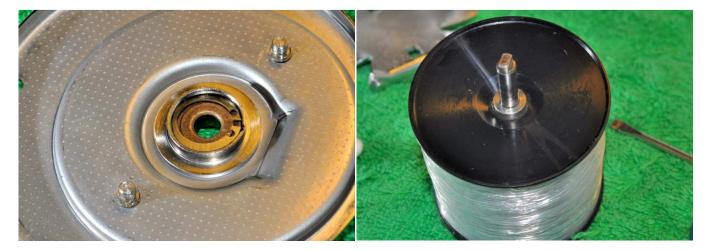
Lubricate the bushing on the left side plate with oil as well as the spool shaft where it contacts the bushings.
