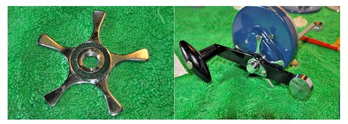
Add some oil to the felt washer underneath the star drag. Replace the star drag and the washer and locking washer. Replace the handle, handle nut, handle nut lock plate, and the handle nut lock plate screw.
