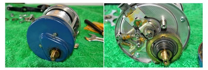
Before opening up the right side plate it is a good idea to remove the left side plate (held in place with three thumb nuts) and the spool from the frame. Remove the star drag and then remove the two bridge screws on the side plate. Remove the side plate.
