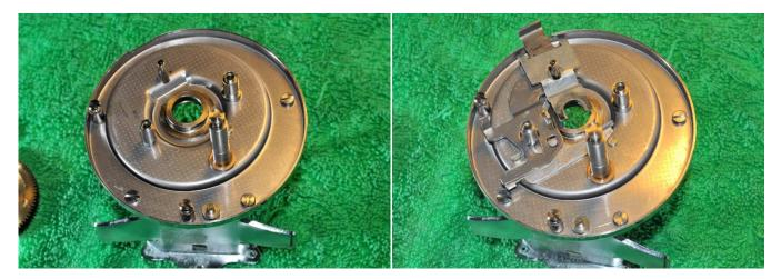
Replace the free spool press arm, free spool clutch and the pinion yoke in the frame applying a light coat of grease to the friction surfaces.
